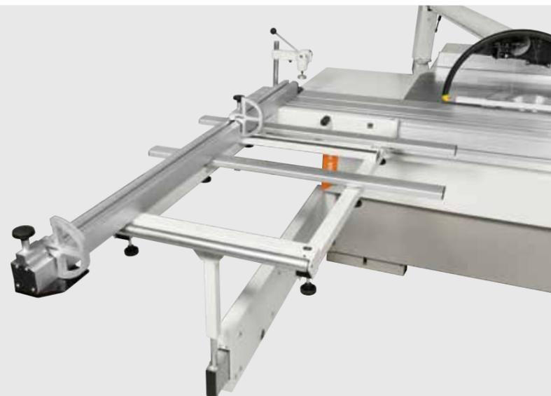
Crosscutting fence with electronic digital readout on every stop (3) with position detecting system of the reversible stops on magnetic band. Available on request.
