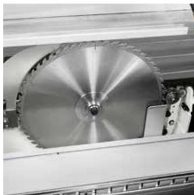
Possibility to equip the machine with 550 mm saw blade without scoring blade installed. (Optional).
