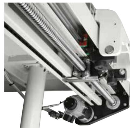
Rip fence with NC positioning, available on request. The fence is positioned by a re-circulating ball screw and it is guided by a prismatic linear way. The fence can be easily flipped over 90° to enable safe ripping of thin and narrow workpieces and can be easily excluded under the worktable. Anti-collision safety system.
