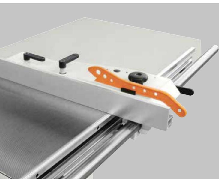
Heavy duty rip fence with micro adjustment through rack & pinion, and fast lock through eccentric pin. The fence slides over a rectified round steel bar and is fully excludable under the table.
