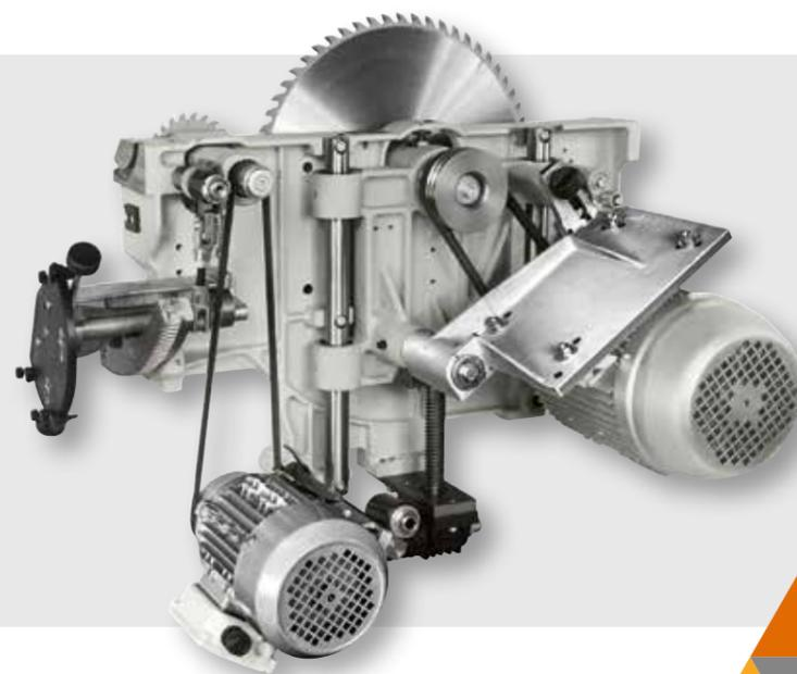
The scoring unit, driven by an independent motor, is micro adjustable through a preloaded system with fast repositioning. Adjustment from control unit for "A" versions.
