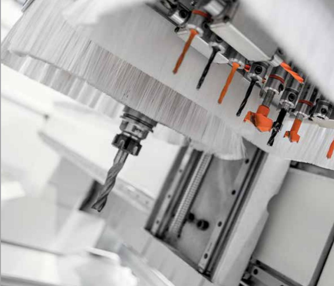
Quick set up with the tool changer LINEAR 11 and ST14 Plus. Possibility to load 25 tools
