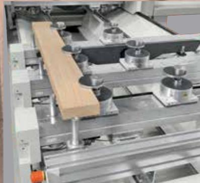
"TL" working table: clamps for machining of solid wood that ensure maximum quality.
