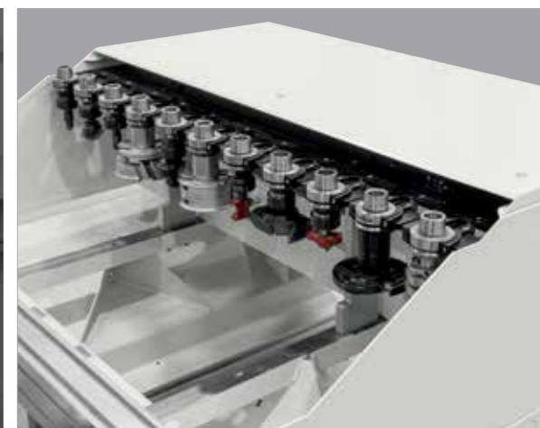
LINEAR 11: linear tool changer on the structure for management of large dimensioned tools.
