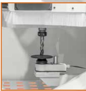
Quick set-up and no errors thanks to the tool length pre-setting device.
