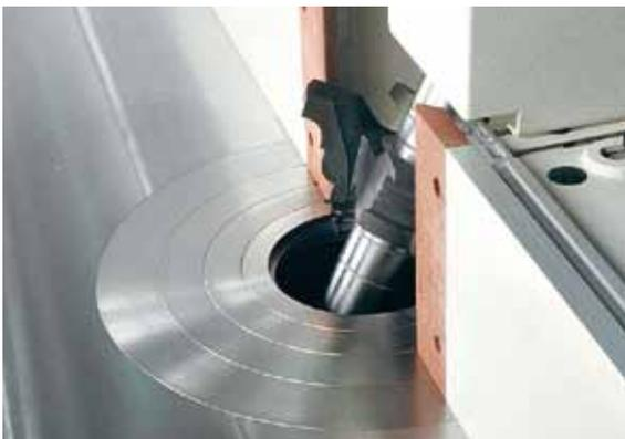
The spindle of the F25, tilting both ways, ensure maximum flexibility.
