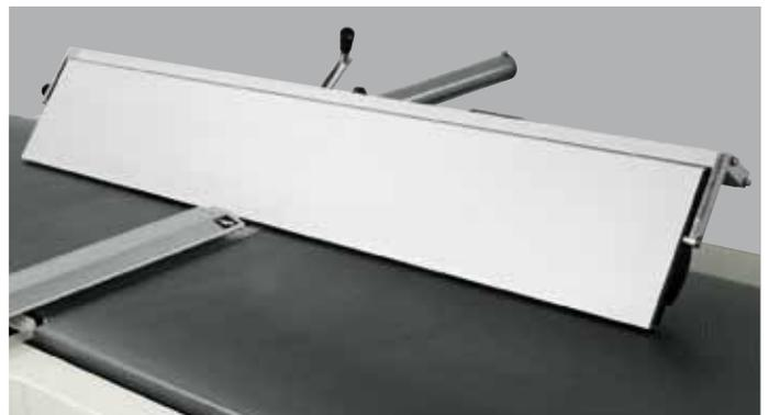
Tilting surface fence  $90^\circ \div 45^\circ$ .
