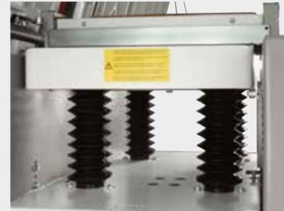
The large dimensioned thickening table is mounted over 4 steel screws protected from the dust. This system is extremely precise and ensures stability even when working long and heavy workpieces.
