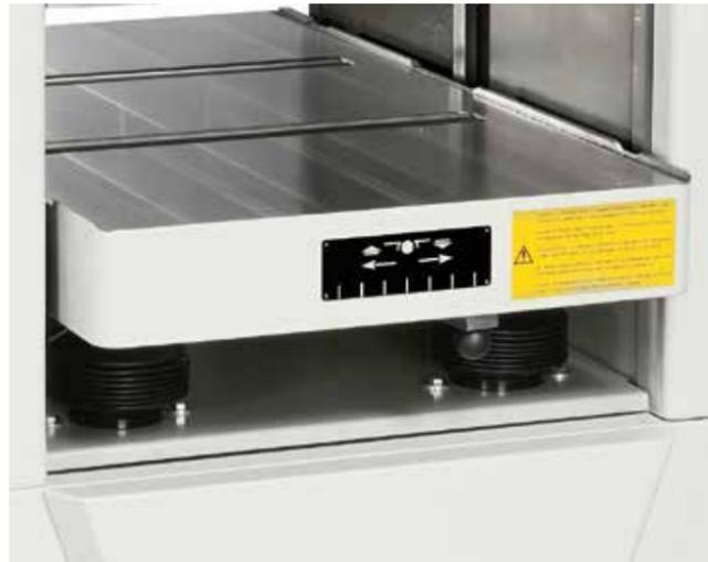
To facilitate feed of large section stock it is available, on request, the worktable with 2 idle floating bed roller with height adjustment.
