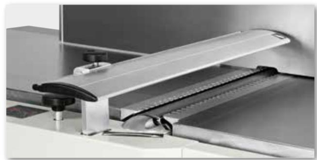
The cutterhead protection ensures the highest safety during working.
