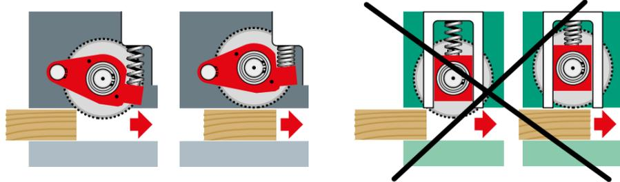
Infeed rollers on independent rods and ball-bushing
