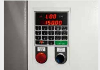
The thickener table electronic positioner, available on request, enables fast and precise worktable positionings.
