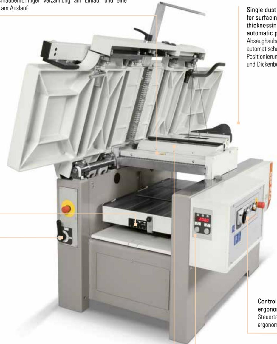
Single dust hood for surfacing and thicknessing with automatic positioning.
