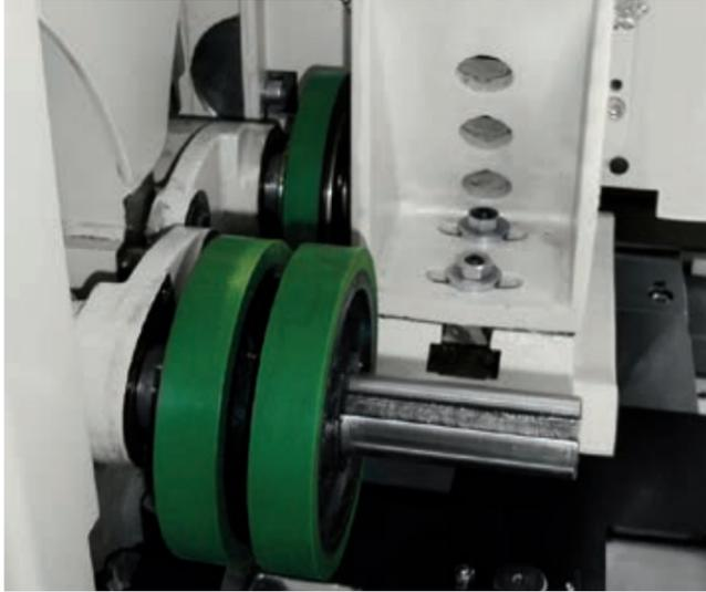
Additional feed unit after top horizontal spindle.
