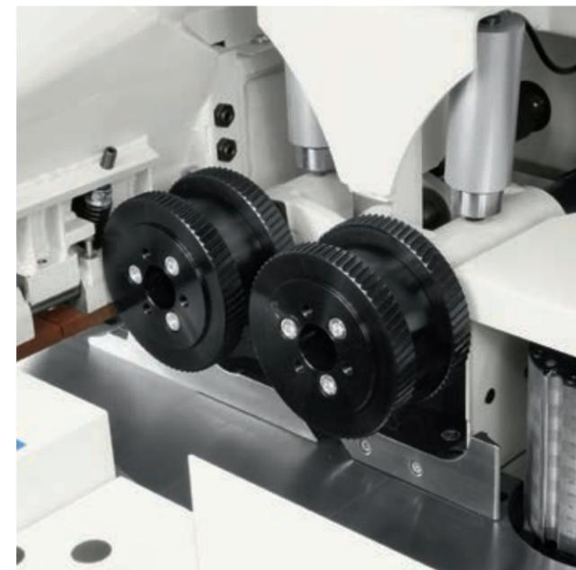
Set of additional front mounting rollers in front of the left vertical spindle.
