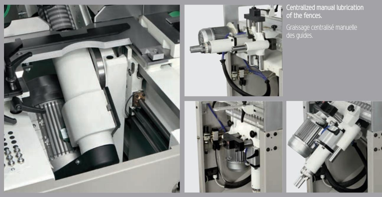
Centralized manual lubrication of the fences.
