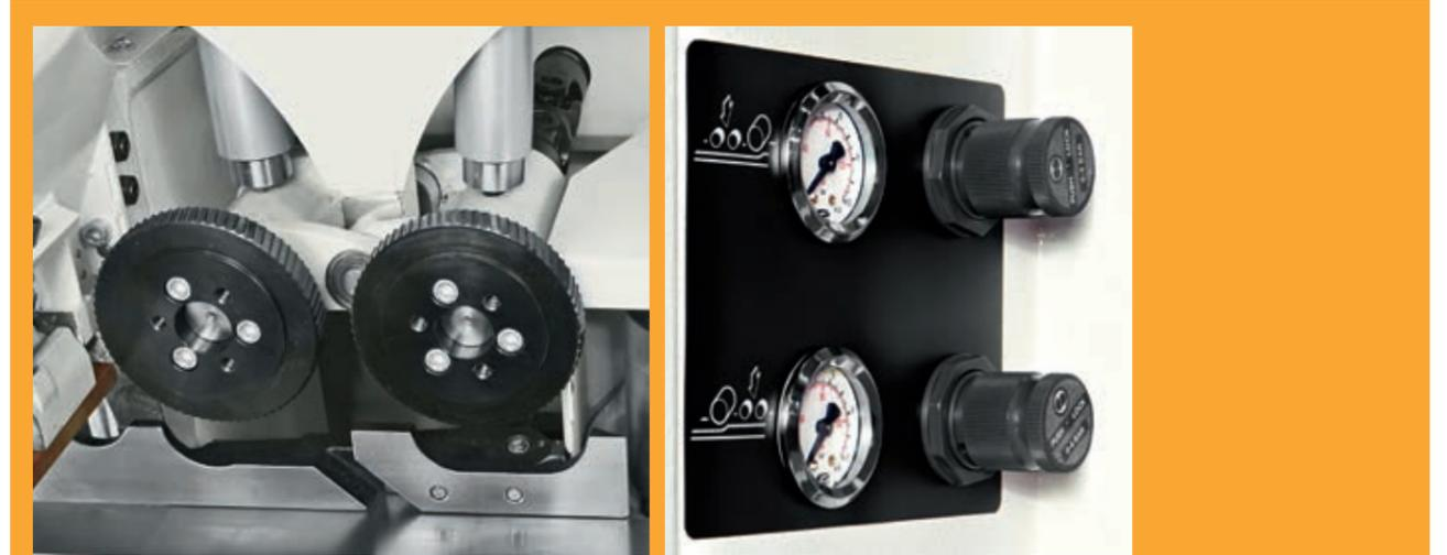
Pneumatic pressure system for the feed rollers.
