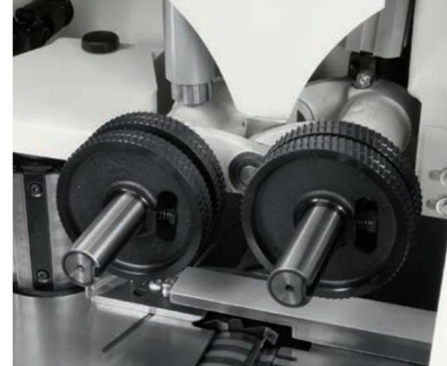
Extra infeed roller unit in front of first bottom spindle.
