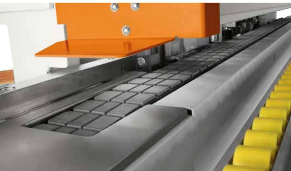
Feeding straightness and resistance to lateral boards thanks feeding system made by chain with of high grip rubber coated pads.
