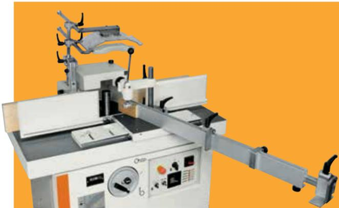
Carriage on main table for small tenoning operations
