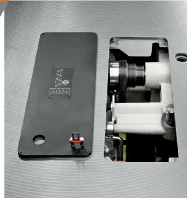
Three saw blade rotating speeds
