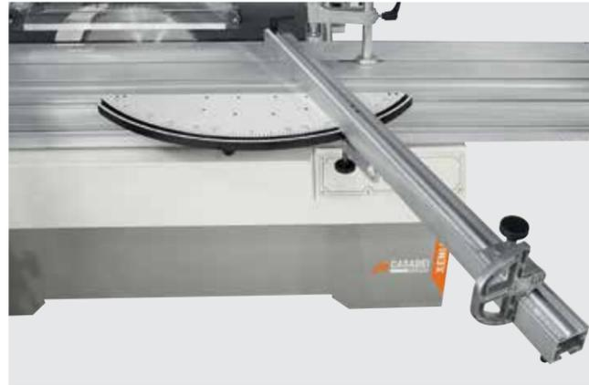
Fence for angular cutting with automatic compensation of the stop position. As the fence is angled the position of the stop remains the same in relation to the main blade: this enables quick set-ups and reduces test cuts.
